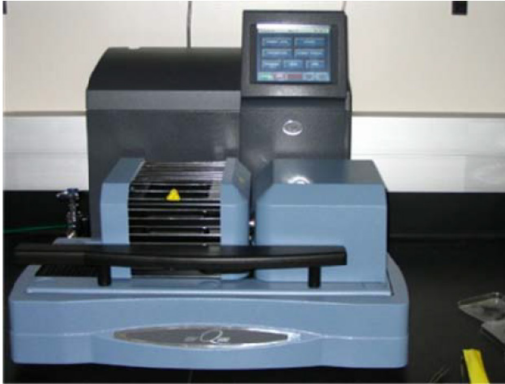
Figure 2.3. TA Instruments SDT Q600, thermogravimetric analysis equipment [140].
