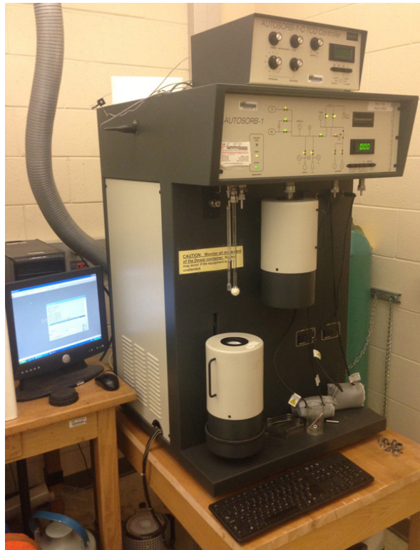
Figure 2.9. Quantachrome AS1C, low pressure volumetric gas sorption tool with chemisorption analysis capability [152]. Quantachrome AS1C is equipped with low pressure transducers ( < 2 atm) to collect high accuracy data at the low pressure region.
