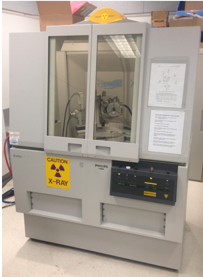
Figure 2.4. Philip X'Pert Pro MD powder X-ray diffraction.
