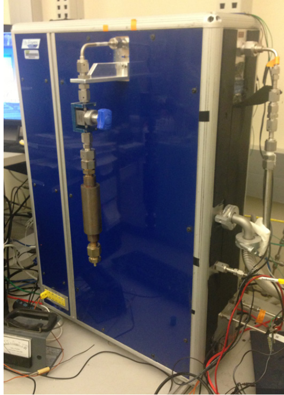
Figure 2.10. Setaram-HyEnergy PCTPro 2000, high pressure volumetric gas sorption tool [153]. PCTPro 2000 is equipped with a high pressure transducer (up to 200 bar) and a heating mantle for high temperature measurements (up to 400 °C).
