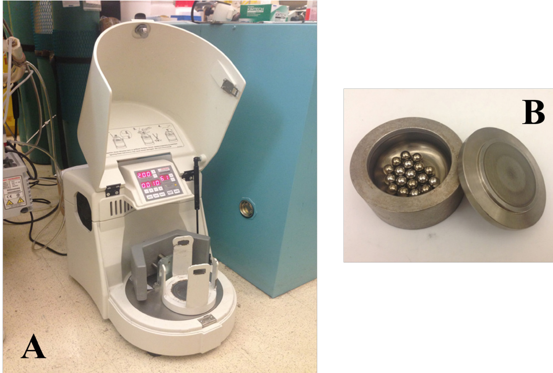
Figure 2.1. (A) Fritsch Pulverisette P6 and (B) 80 ml stainless steel bowl, lid and \text{\O} 10 \text{ mm} stainless steel balls [136].
