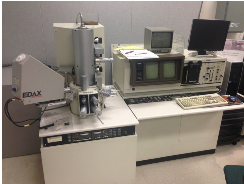
Figure 2.5. Hitachi S-800 scanning electron microscope.
